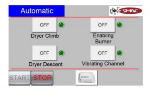
Automatic page, where we can include or exclude some of the utilities from the automatic cycle. We also have the command to bring up or down the dryer.
