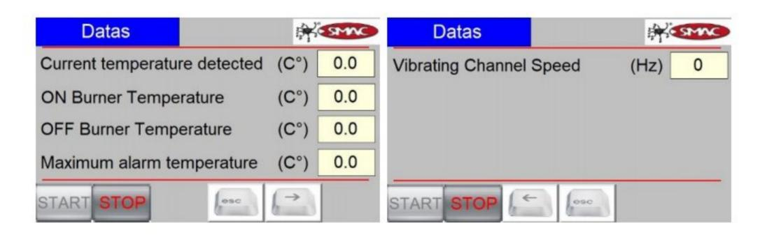
Data pages to set for automatic machine operation. Press ESC to return to the main menu.
