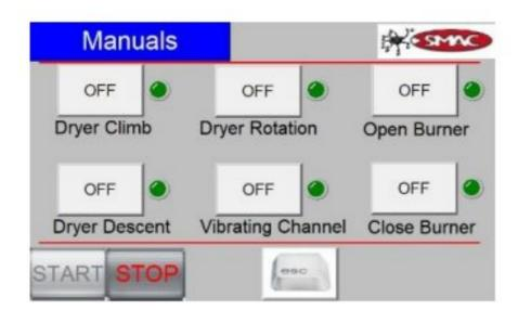
Manual controls page where you can select the user you want to activate by pressing directly on the corresponding button. It is also possible to view the status of the various utilities during any operation (manual or automatic) through the ball next to each key that will turn on when the user will be in operation.
