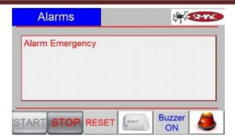
Press the "Buzzer ON" button to mute the audible alarm. In the page of active alarms we can have several alarms.
