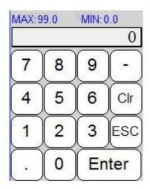
Every time a data is called, a keyboard will appear to enter the value. On the keyboard will be indicated in addition to the value entered also the minimum and maximum value that the data may have.
