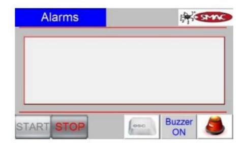
Pressing the reset button the page will have to present itself as above. This will indicate that there are no other active alarms and therefore the machine is ready for operation.
