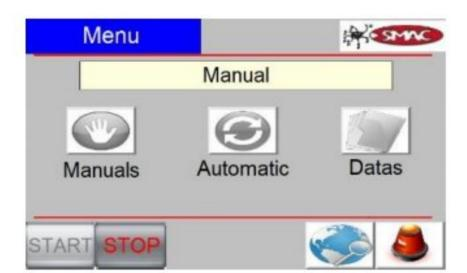
In case of an alarm, a button will appear on the touch-screen, in addition to the written alarm, as a visual signal at the bottom right representing a flashing light. By pressing the button you will have access to the page of active alarms.
