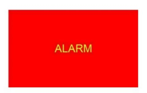
When an alarm appears the alarm window will appear as above, clicking on it will disappear and the alarm summary window will appear, if the alarm is not reset within 20 seconds the pop-up will recur.
