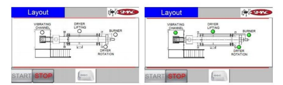
The page appears 20 seconds after the machine is in automatic mode. Layout page where it is possible to view the status of the various utilities during operation.
