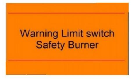
This page appears when the burner is opened and the safety micro is triggered, which will extinguish the flame. Pressing on this page the latter will close but if we have not closed the burner will reappear after 20 seconds.
