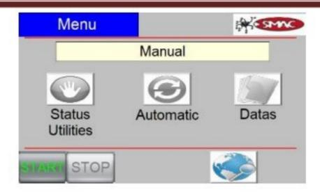
In case of machine in Automatic (AUT), the manual controls button changes name because in this mode we can only view the various users if they are active and we can not use manual commands.
