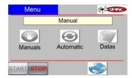
Main menu with machine in Stop where we have at the top the machine status (Manual, Automatic, etc.), the button for selecting the language page (bottom right), the button for selecting the manual command page, the button for selecting the automatic cycle page and the button for selecting the data page.
